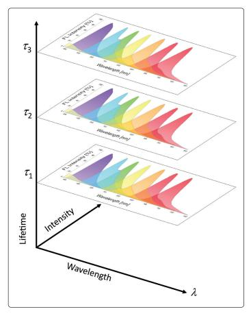
TRFC has the capability to triple the number of colors for each detector and can enable 8–12 colors per laser—or 40+ colors with 5 lasers with a greatly simplified workflow.
