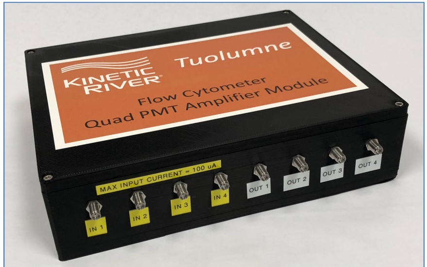
The Tuolumne is a compact (9" x 8.5" x 3") quad port PMT amplifier module for use in flow cytometry applications
