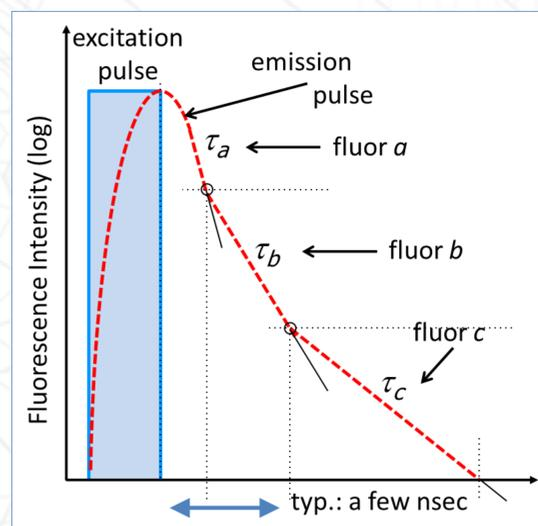
Figure 2. Direct time domain measurement of fluorescence lifetime enables discrimination of multiple fluorophores simultaneously. Note the multi-exponential decay curve.
