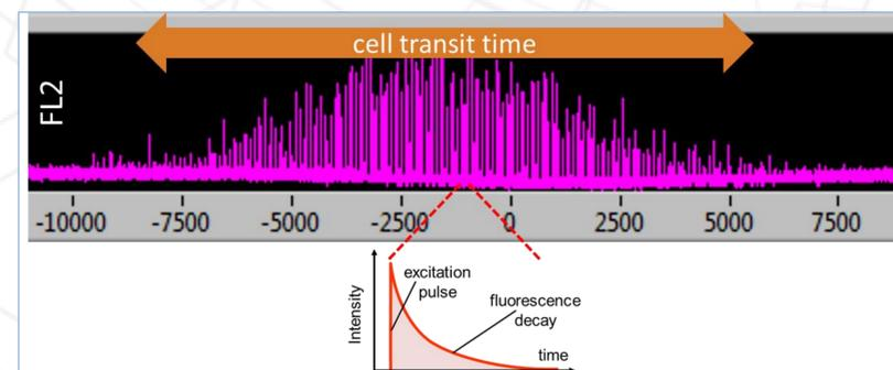
Figure 1. Whereas continuous laser excitation in conventional flow cytometry yields a single intensity value per event, time-resolved fluorescence pulses excitation light hundreds of times per event, each pulse yielding a decay curve measured during the off period. Each fluorophore has its own characteristic decay lifetime.
