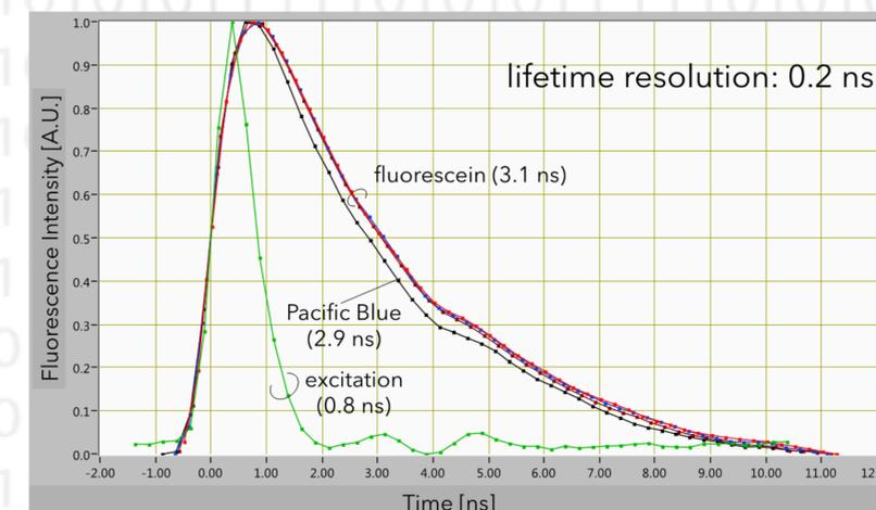
Figure 6. The Danube provides lifetime resolutions as low as 200 psec. Like FLIM, lifetime measurements in flow can be used to detect changes in the cellular microenvironment of the fluorophore, which can alter lifetimes. This enables assays of changes in protein conformation, protease activity, receptor ligand interactions, pH and calcium concentrations, and more.
