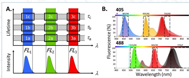
Figure 3. A) By multiplexing in the lifetime parameter, 3 separate fluorophores (a, b, and c) may be detected in each channel (FL1, FL2, and FL3) simultaneously. B) A 12-color, compensation-free Arno design uses two lasers (405 and 488 nm) and six detectors, with two spectrally overlapping fluorophores detected in each channel.
