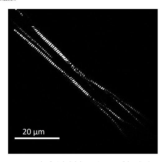
In this microscopy image, myosin bundles (individual white spots) in a stem-cell-derived cardiomyocyte stand out against the background due to their intrinsic, label-free second-harmonic generation (SHG) signal. Courtesy
