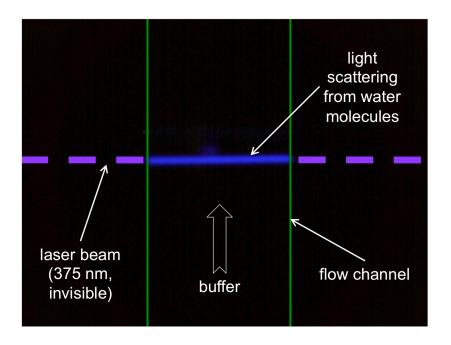
The *Tiber* technology is based on a pulsed UV laser for label-free excitation of biomolecules. The laser beam, which invisible to both the eye and most cameras, shows up in this image as deep blue due to Raman scattering from water molecules in the flow channel of the *Tiber* instrument. The instrument sensitivity is such that this normally undetectable signal has to be specially filtered out.
