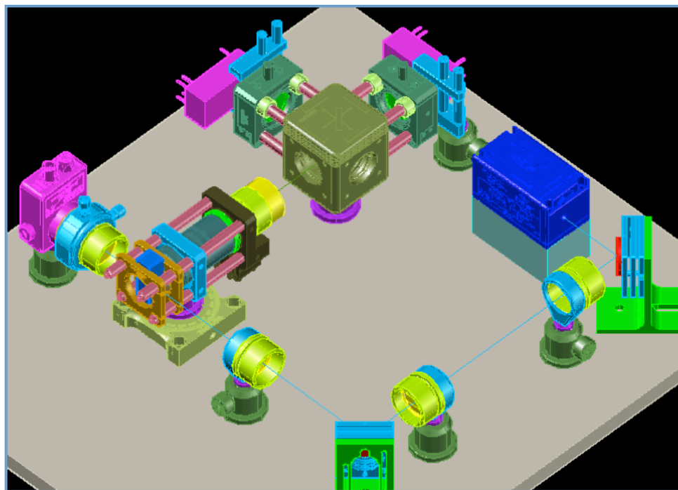
Figure 3. Automatically generated BeamWise 3D CAD rendered drawing of the flow cytometer optofluidic bench.
