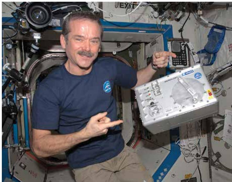
**Figure 5.** Canadian Space Agency astronaut Chris Hadfield, floating in the International Space Station, together with INO's Microflow cytometer. The instrument was tested on the space station to pave the way for health monitoring of astronauts during space missions.
