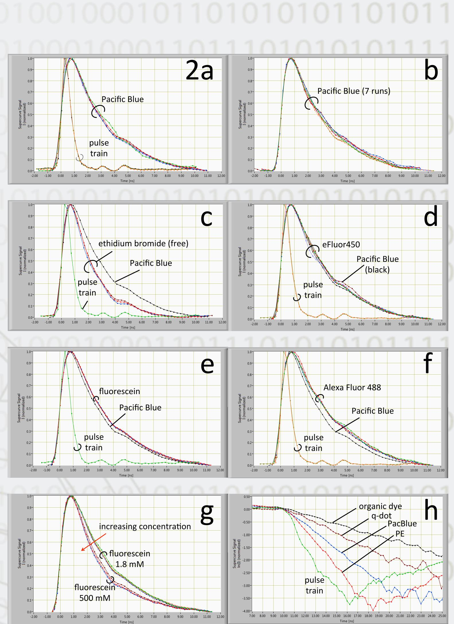
Direct time-domain capture of fluorescence lifetime is a viable and highly accurate approach to reliably quantify multiexponential decays in flow. Based on our Danube instrument platform, we are currently designing a next-generation instrument architecture that will be capable of high-throughput analysis with real-time lifetime extraction, ultimately suitable for sorting applications.
