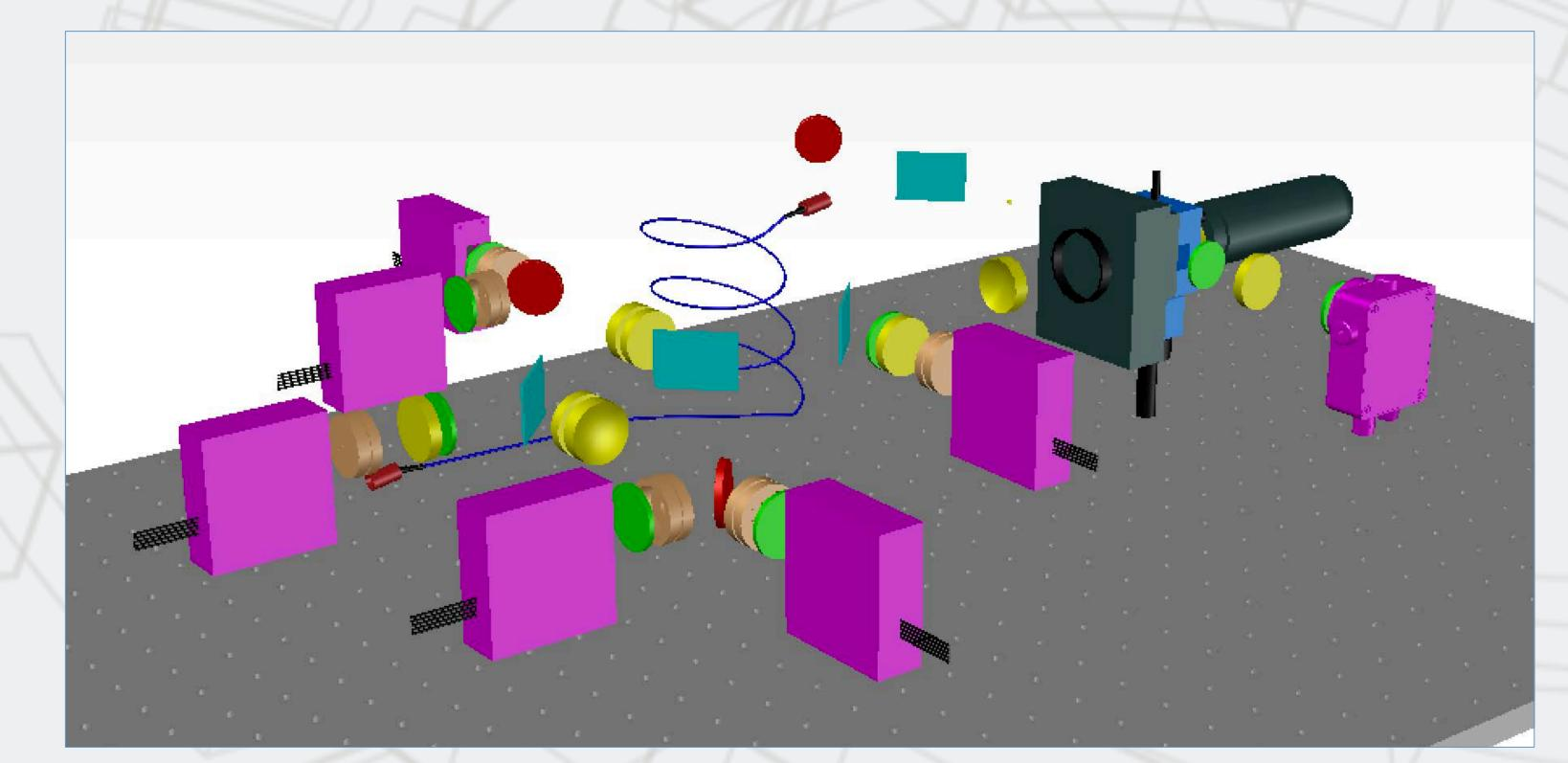
We have developed a new platform for flow cytometry, the *Potomac*, to serve the unmet need of an open and flexible architecture for cell analysis. This platform is the result of a complete from-the-ground-up design effort by Kinetic River Corp. to satisfy the requirements of the National Cancer Institute. The architecture can support up to 7 lasers and 20 detectors, and can be completely customized in terms of light sources, fluidics, filters, and detectors.
