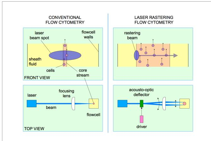
Over the last several years, researchers at Abbott Laboratories have been building and perfecting laser rastering flow cytometry. Three features distinguish laser rastering from conventional flow cytometry: instead of a single line of cells, a wide stream is used; instead of a broad elongated spot, a tighter laser spot in both dimensions is utilized; and, finally, the laser beam is scanned or rastered across the core stream as the cells go by.
