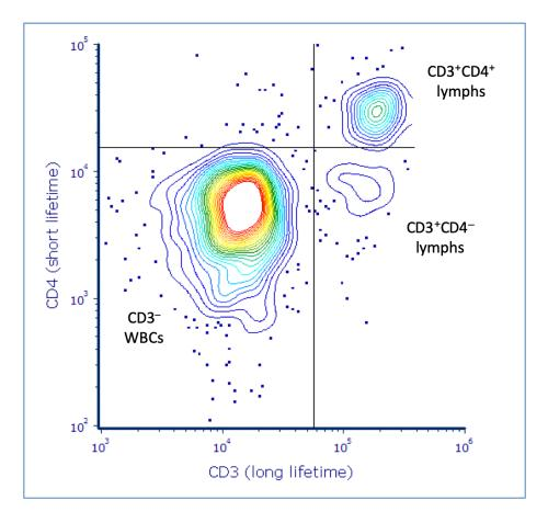
Data from lyophilized white blood cells (WBCs) obtained on the *Arno* platform. The signals corresponding to CD3 and CD4 expression in lymphocytes were collected simultaneously by a single detector, and are easily discriminated solely based on the lifetimes of the respective fluorophores despite their completely overlapping emission spectra. Copyright © 2019 Kinetic River Corp.
