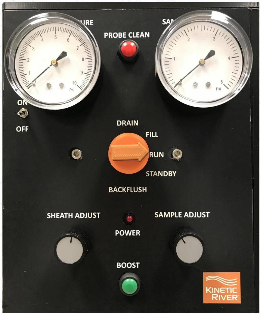
Figure 1. The Shasta Fluidics Control Module front panel with all-analog dials and gauges.
