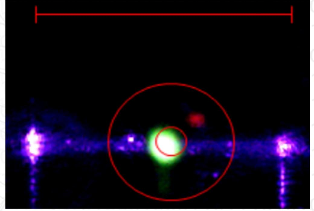
Figure 3. Core stream generated using the Shasta (fluorescein excited with a 405-nm laser). Bar = 404 µm.
