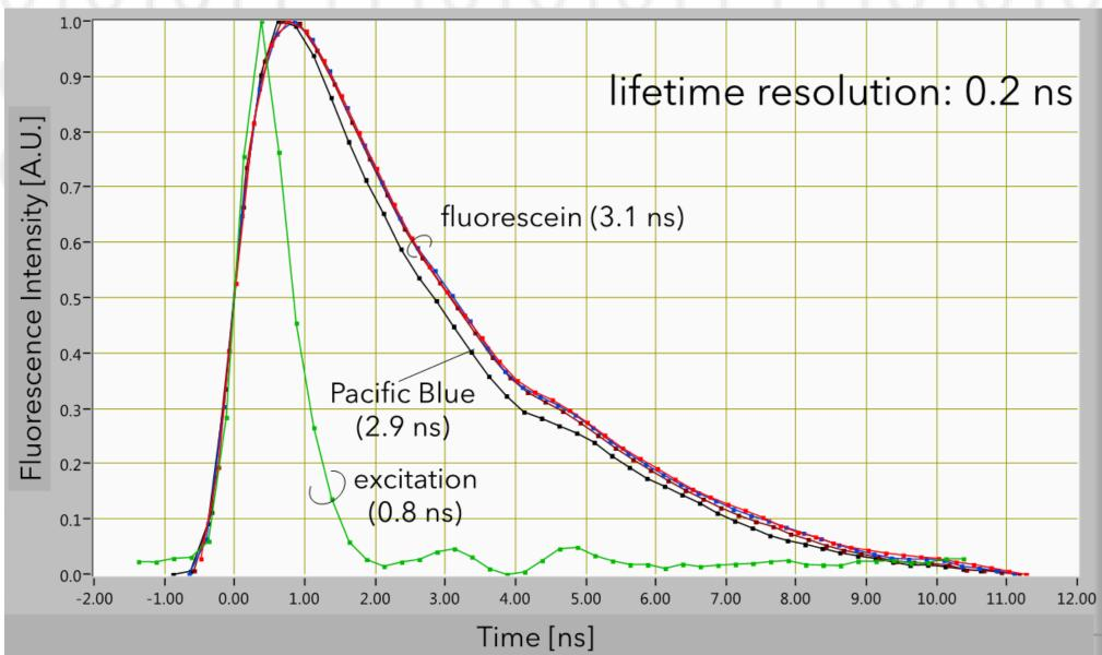
Figure 6. The Danube provides lifetime resolutions as low as 200 psec. Like FLIM, lifetime measurements in flow can be used to detect changes in the cellular microenvironment of the fluorophore, which can alter lifetimes. This enables assays of changes in protein conformation, protease activity, receptor ligand interactions, pH and calcium concentrations, and more.
