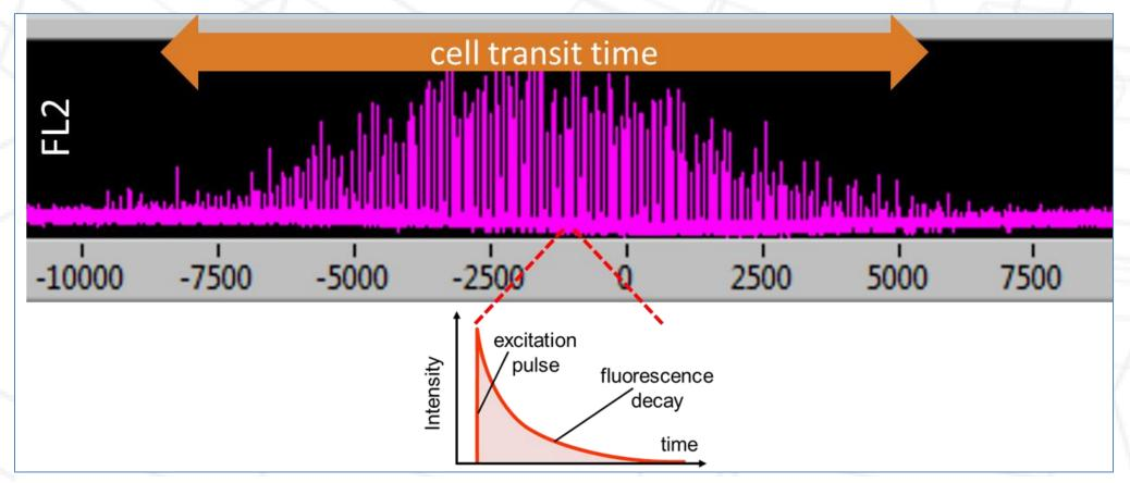
*Figure 1.* Whereas continuous laser excitation in conventional flow cytometry yields a single intensity value per event, time-resolved fluorescence pulses excitation light hundreds of times per event, each pulse yielding a decay curve measured during the off period. Each fluorophore has its own characteristic decay lifetime.
